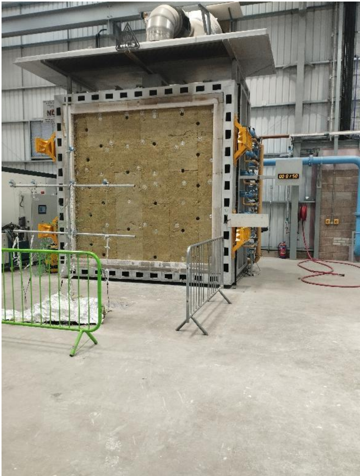
Photograph 11 – Sample on the furnace before the start of the test.
