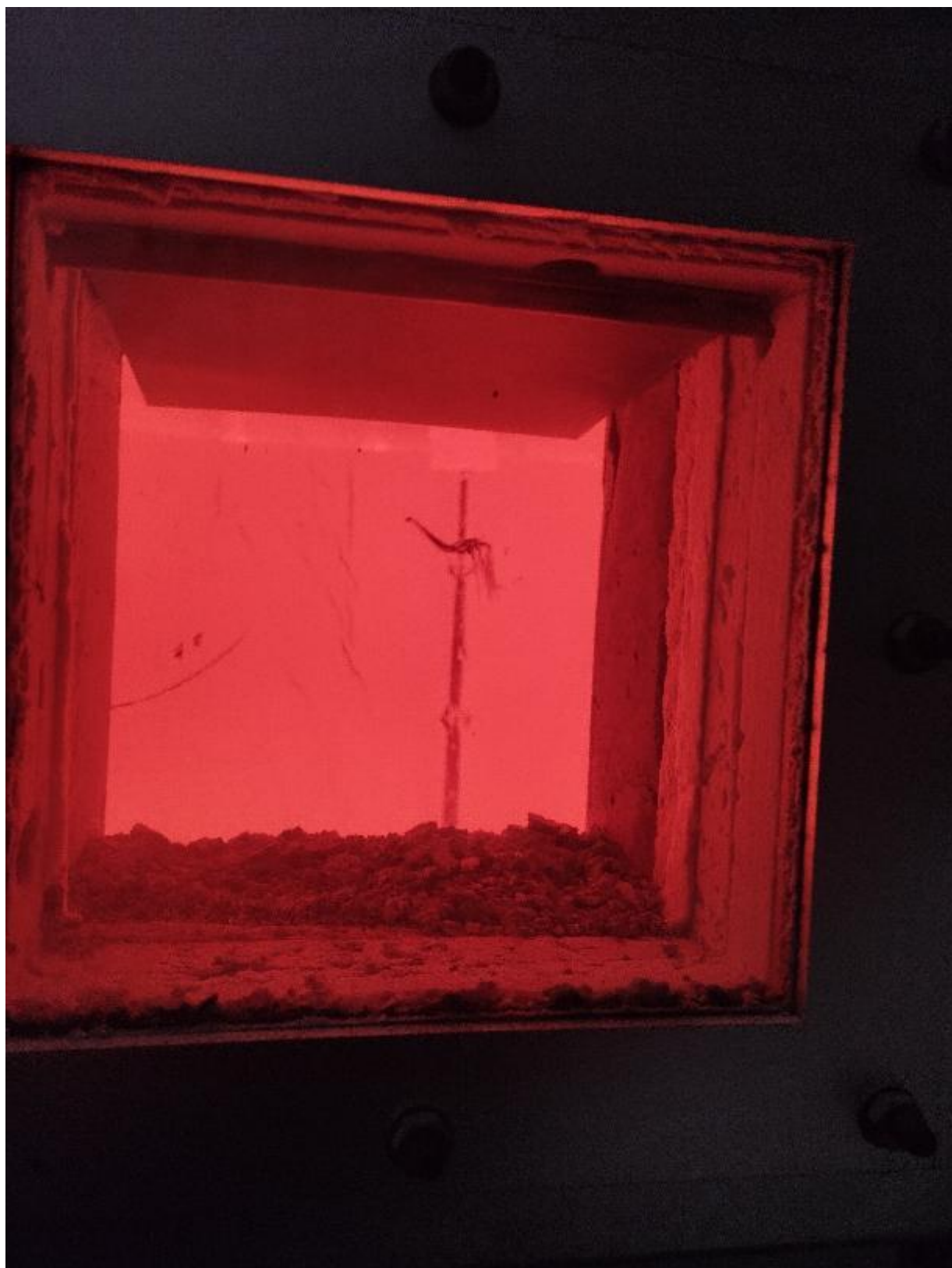
Photograph 22 – Exposed side at minute 90, large gaps between joints
