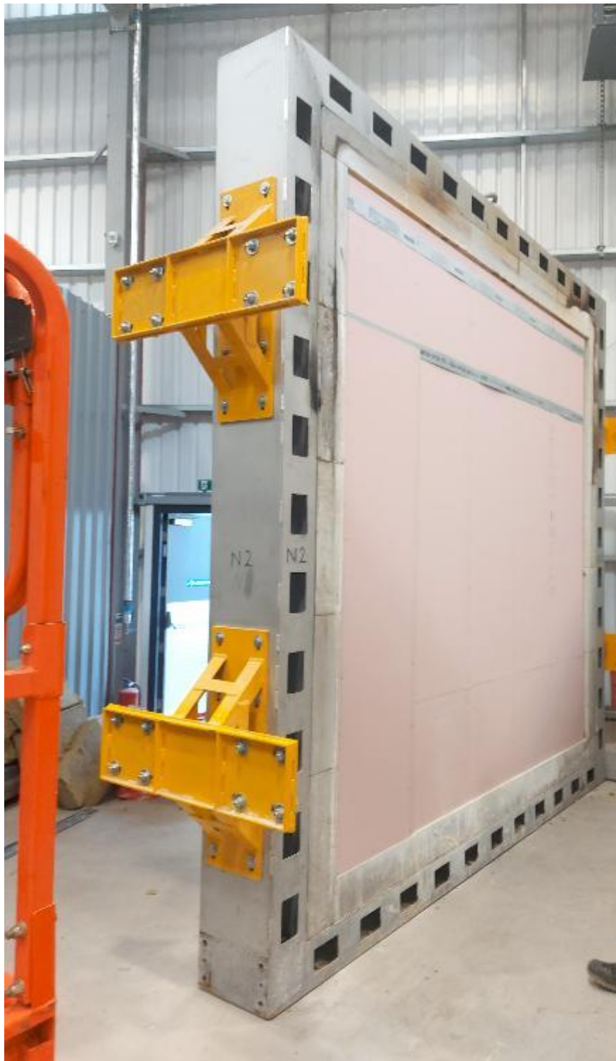
Photograph 5 – First layer of plasterboard on fire side
