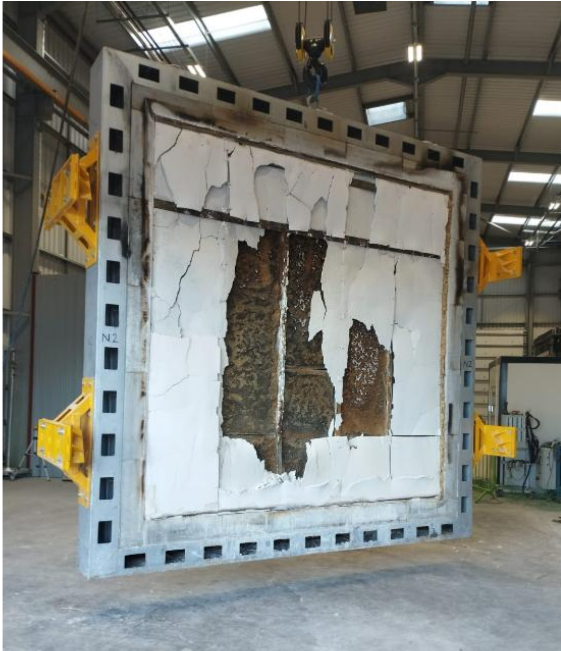
Photograph 25 – Fireside of the sample after the test
