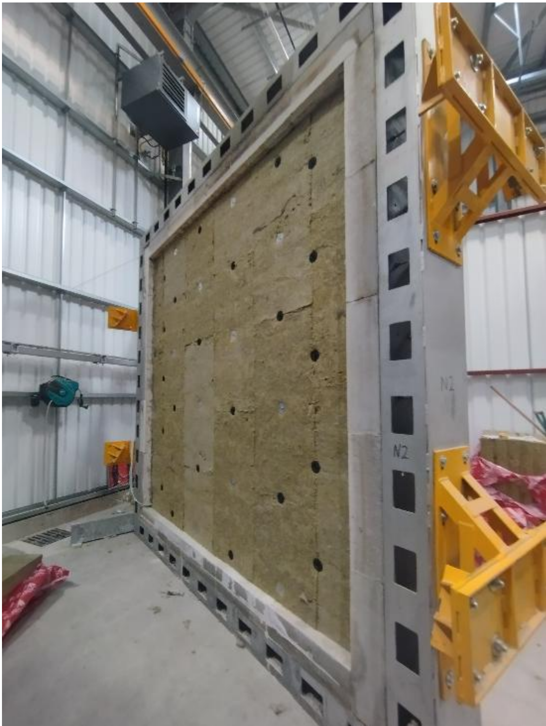
Photograph 10 – Insulation fitted on non-fire side.
