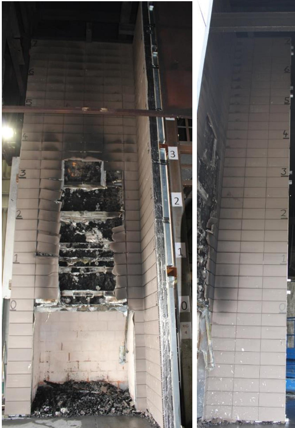
Figure 51. Full-height photograph of cladding system immediately after test.
