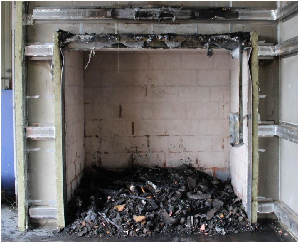
Figure 56. Photograph of the horizontal cavity above combustion chamber.
