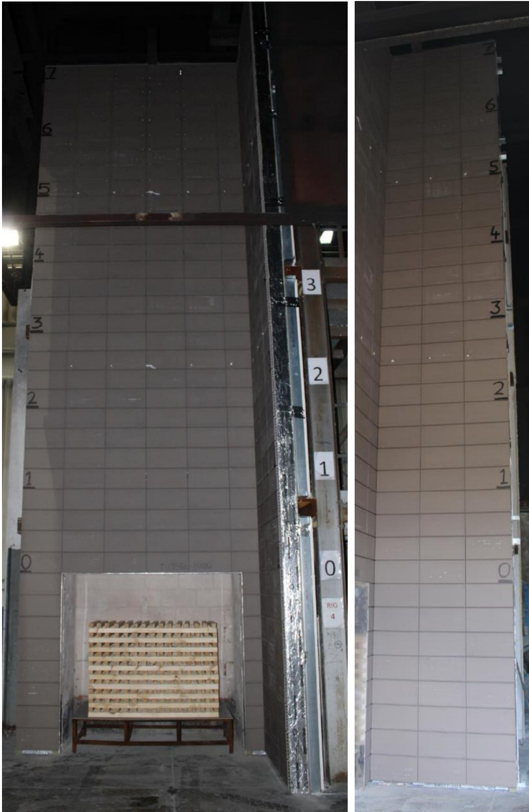
Figure 35. Full-height photograph of completed installation prior to testing.
