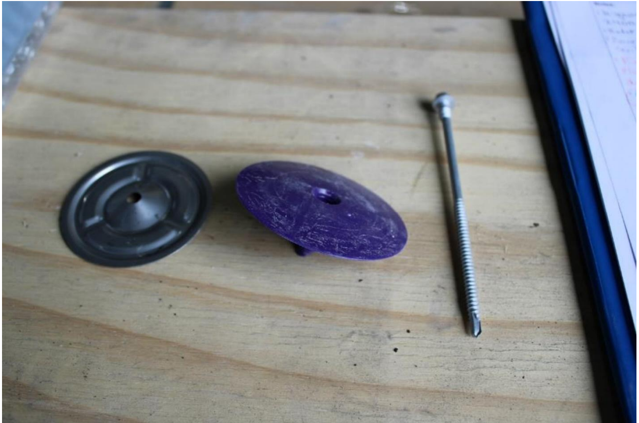
Figure 14. Insulation fixing washers and screw.
