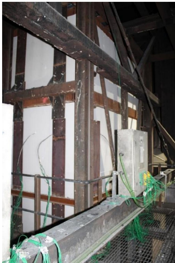
Figure 65. Post-test photograph of the plasterboard (unexposed face) – Level 2 thermocouples.
