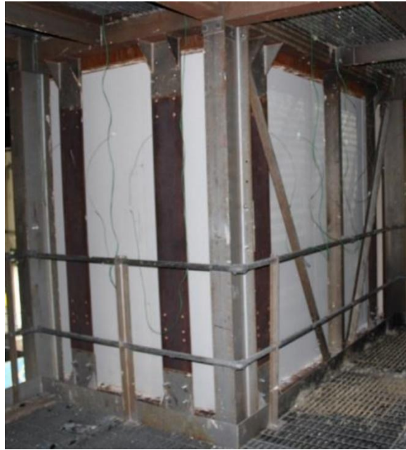
Figure 64. Post-test photograph of the plasterboard (unexposed face) - Level 1 thermocouples.
