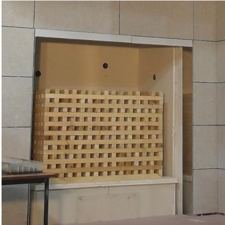
Figure 4.1. Wood crib used on the tested façade – dimensions of the opening are shown.
