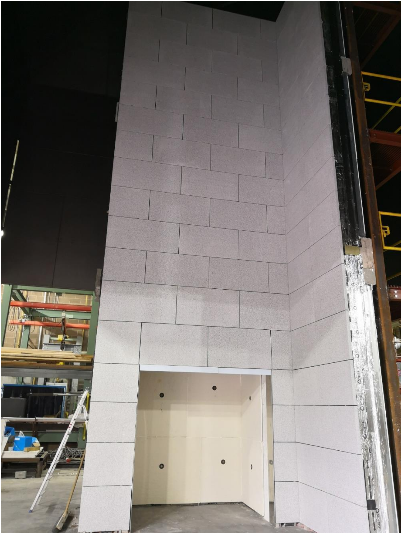
Figure 4.8. Cladding system before test.
