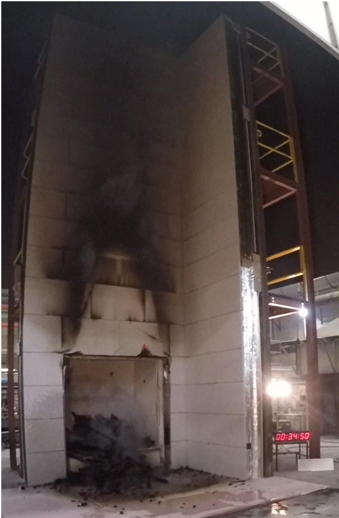
Figure 4.13. Cladding system after fire extinguishment (34 min 50 sec after ignition of the crib).
