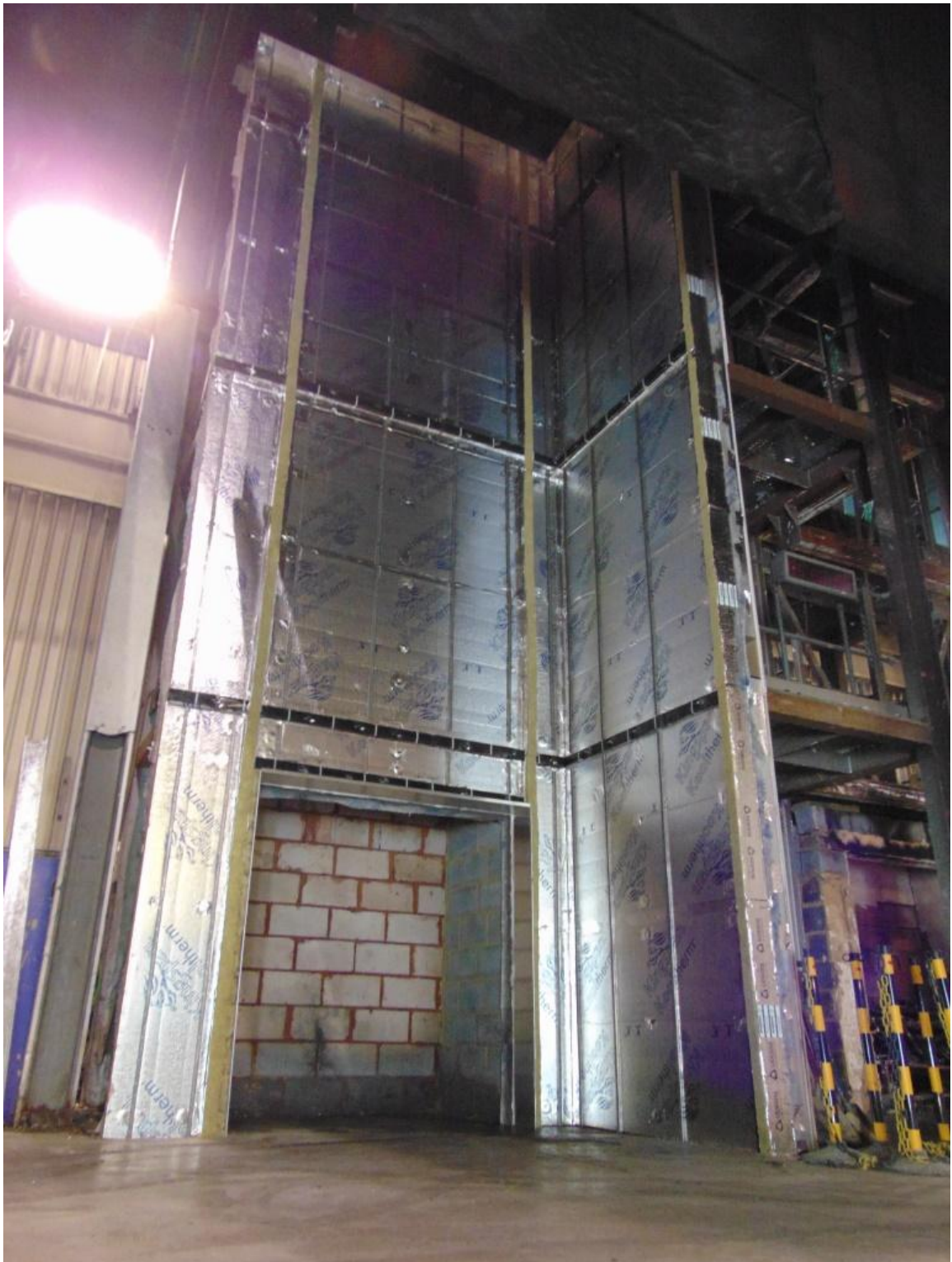
Figure 6. Cavity barriers, insulation and rails.
