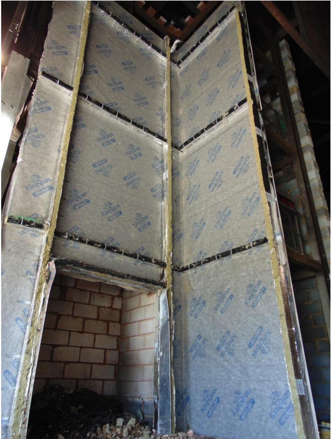
Figure 28. Photograph of horizontal and vertical barriers after test.
