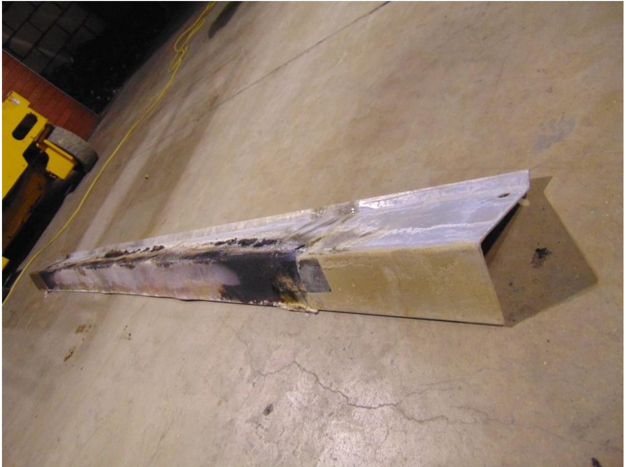
Figure 25. Photograph of steel lintel after test.
