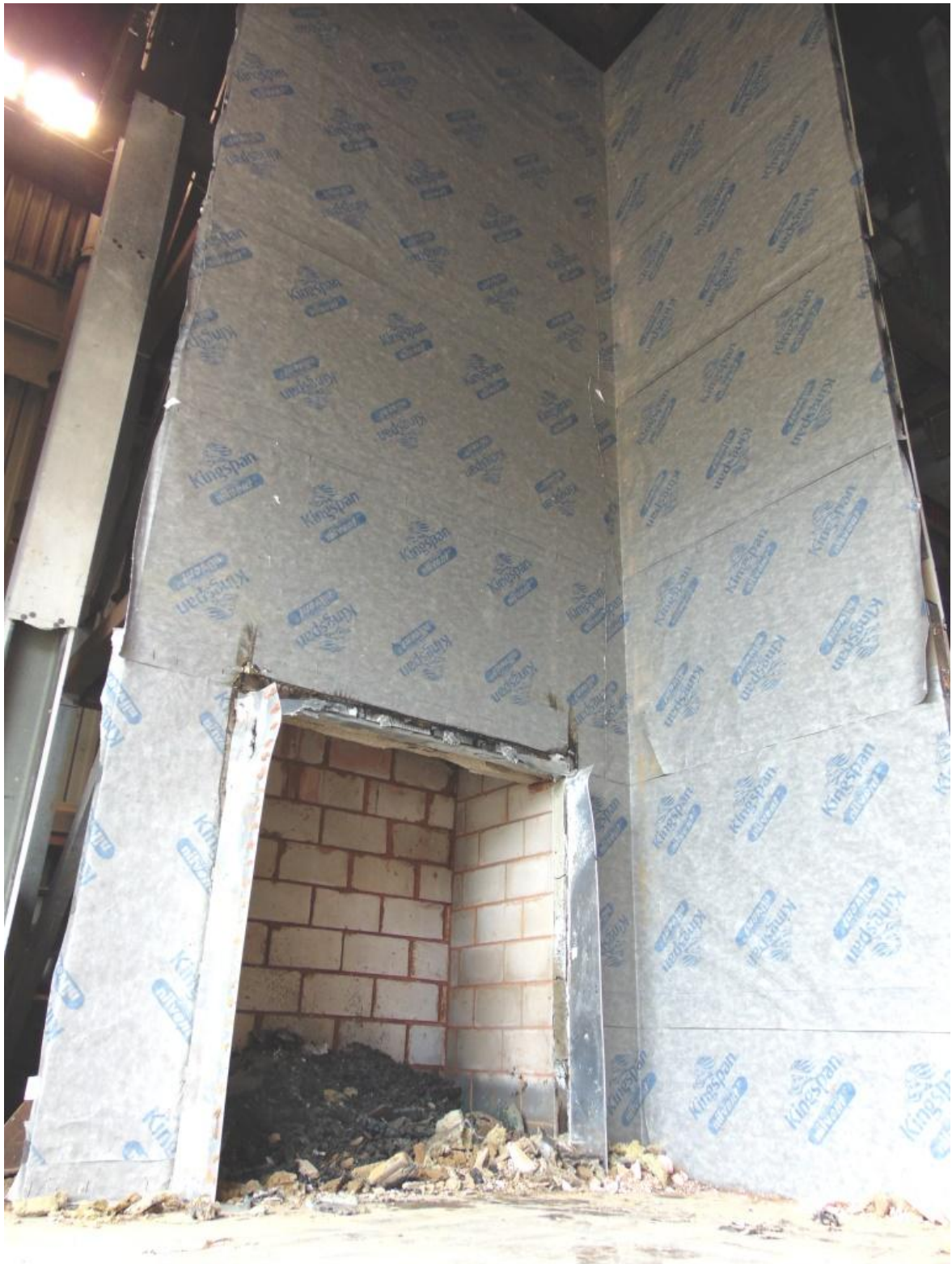
Figure 29. Photograph of breather membrane after test.
