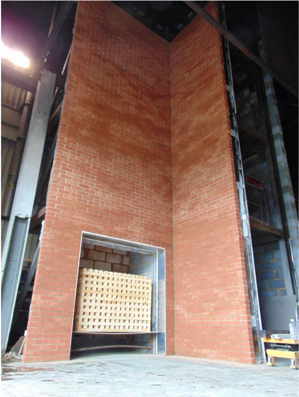
Figure 8. Full-height photograph of cladding system prior to test.
