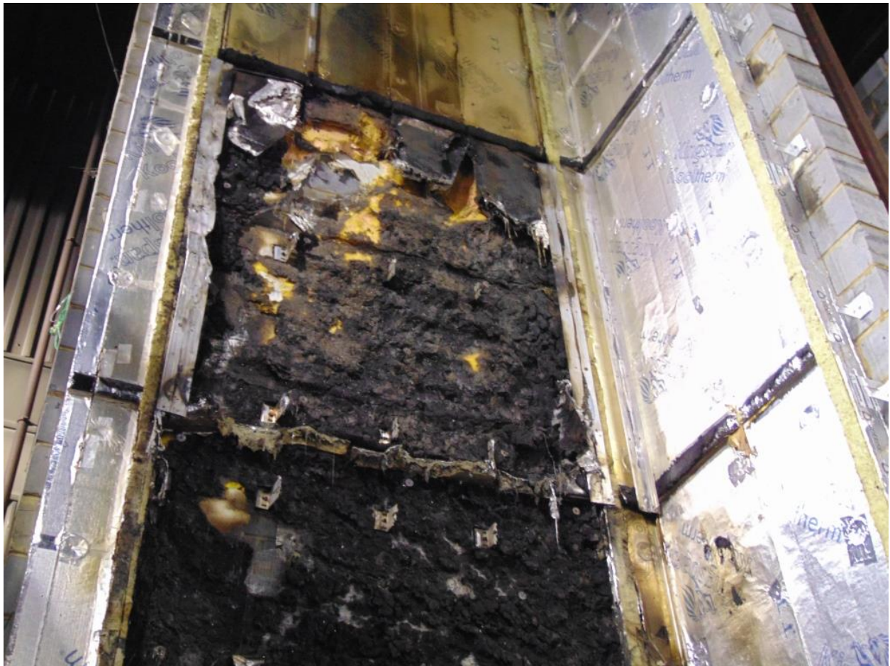
Figure 18. Post-test photo between second and third row Siderise RH25G 90/30 horizontal open state cavity barriers.
