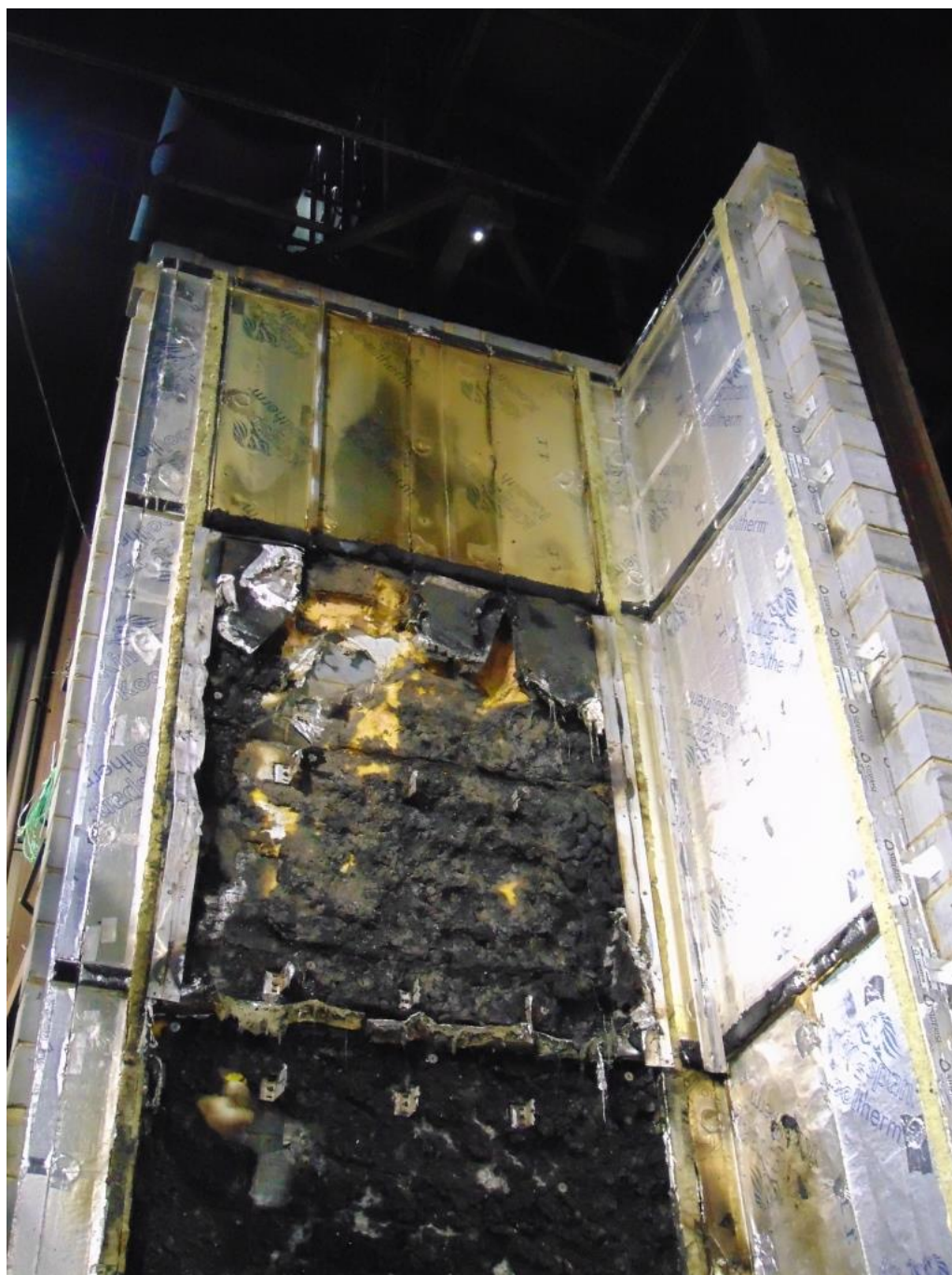
Figure 17. Post-test photo of system following removal of cladding panels.
