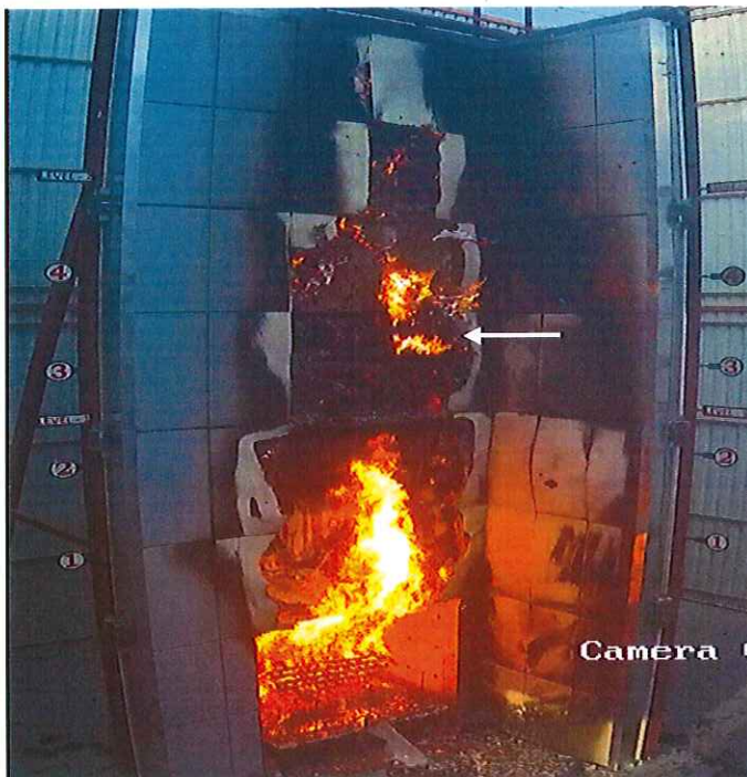
DLP C2753J/0010 Flaming debris of the insulation behind panel M24.
