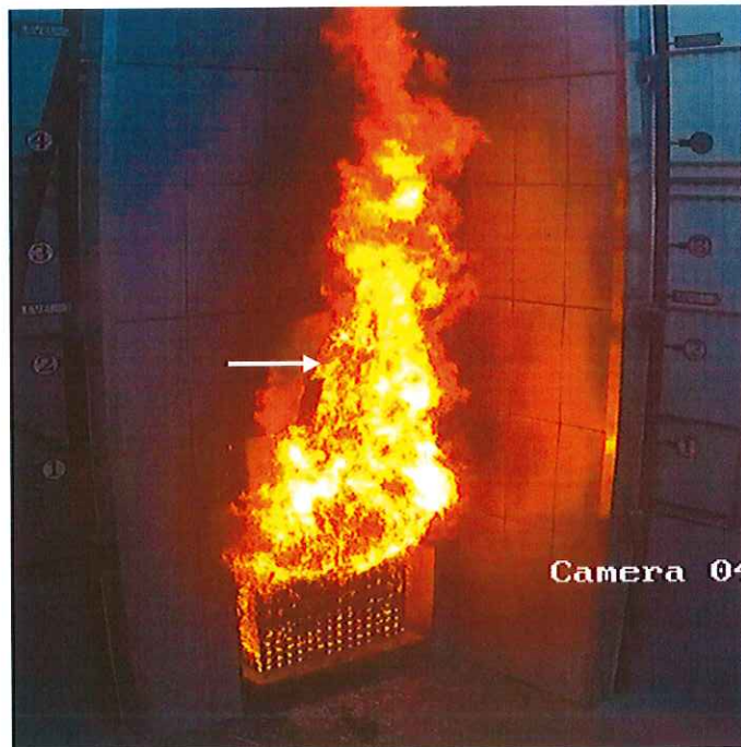
DLP C2753J/0002 Panels M9, M10, M14 & M15 partially melted and insulation behind the panels burning.
