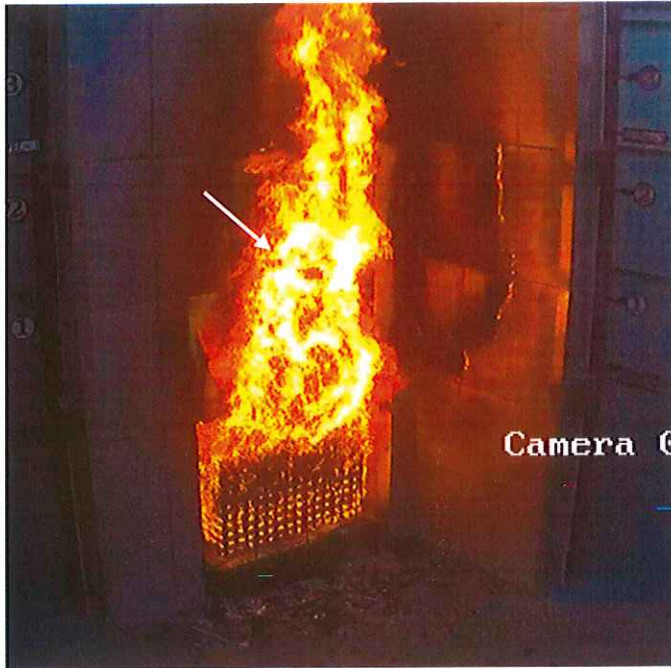
DLP C2753J/0005 Approximately 90% of panels M9, M10, M14 & M15 melted.
