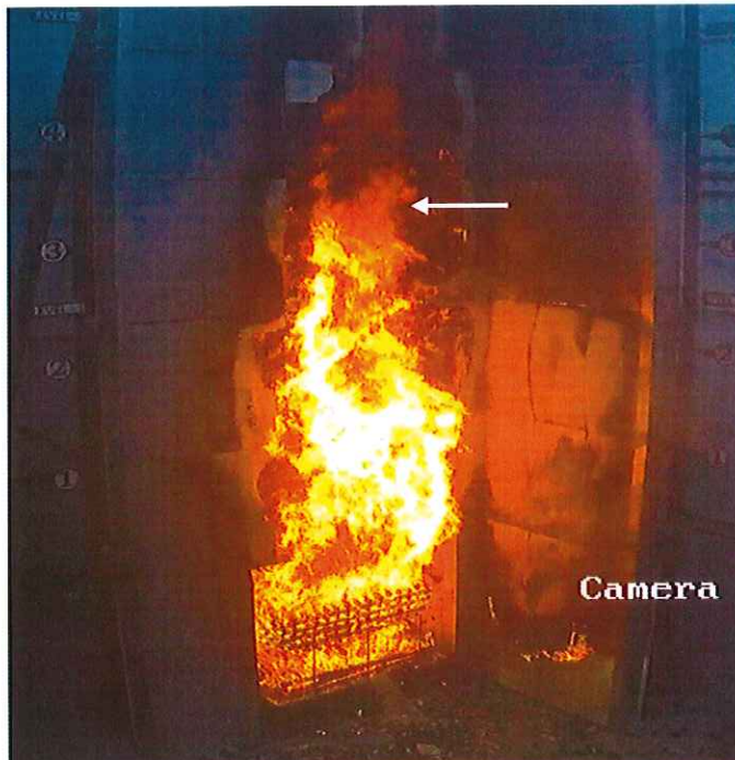
DLP C2753J/0008 100% of the panels M19, M20, M25 & M30 consumed fell off.
