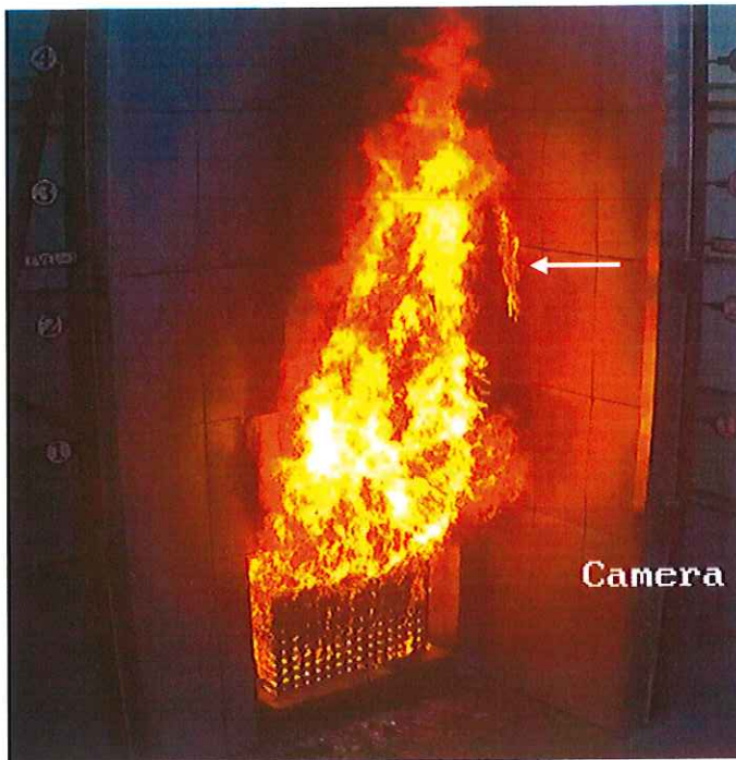
DLP C2753J/0003 Self-sustained flames on the surface of panel W7.
