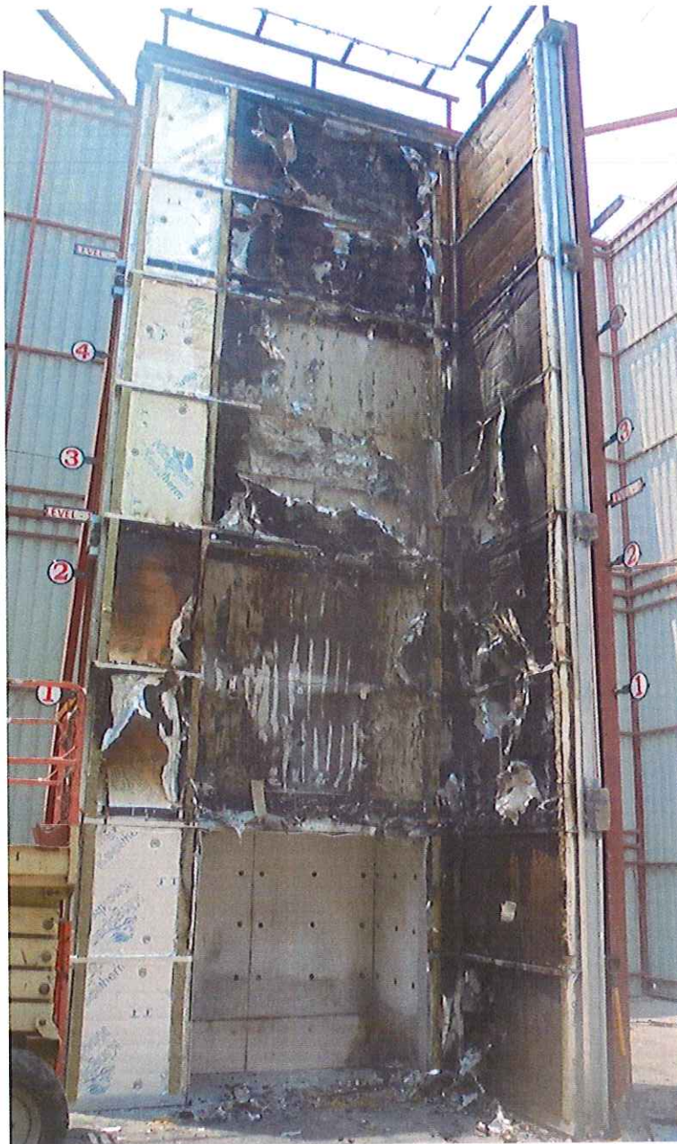
Kingspan Kooltherm K15 insulation, cavity barrier and railings
