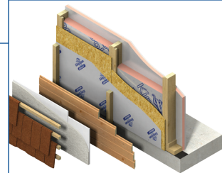
Insulation for timber and steel framing systems
