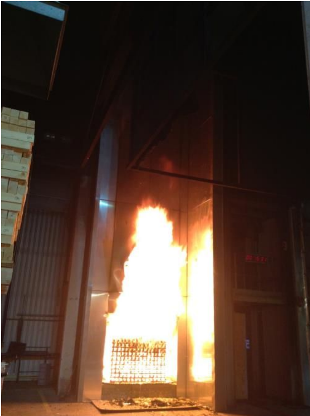
Figure 17. Cladding system during the test.
